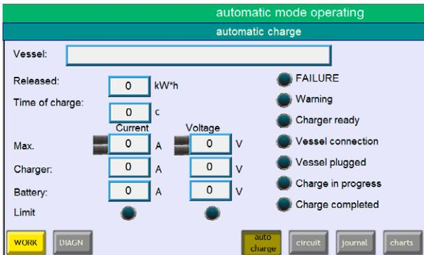
The main screen displays key information on the charge: charge time, amount of supplied electricity, current and voltage set points, and their current values, vessel identifier, system status overview.
